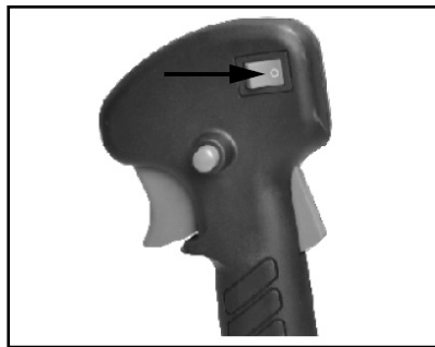
8. If meet any problems, press the engine stop switch, the machine will stop running. If need stop cutting head working, release the throttle lever.
