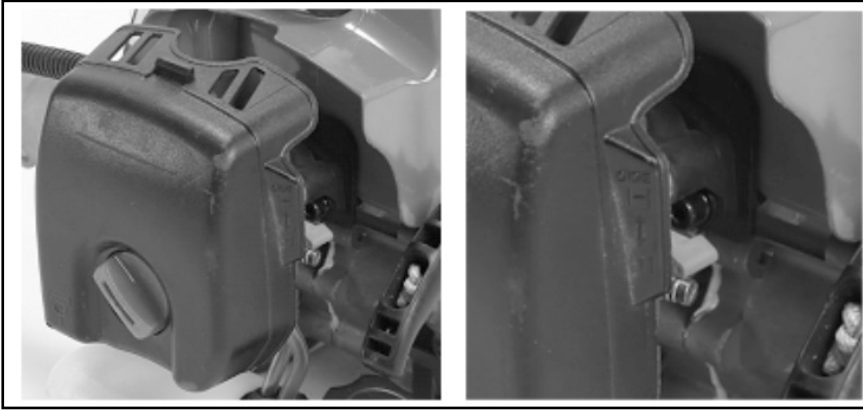
3. Put the choke lever on the OFF position
