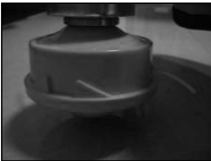
7. If use Nylon cutter, before cutting, need bump to feed line on hardness area
