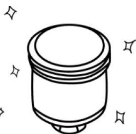
Remove the fuel filter cup. (Model: Simple unit)
